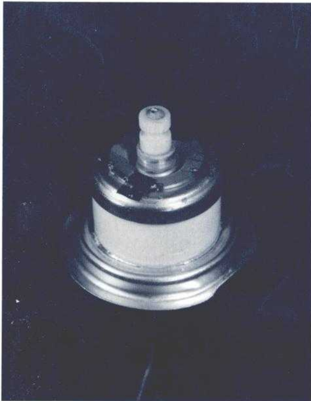
Figure 11. Ceramic insulators typical of those tested to determine resistance to voltage breakdown
