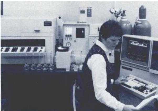
Figure 6. Inductively coupled plasma emission spectroscopy system used for quantitative analysis of elements in concentration down to a few parts per billion
