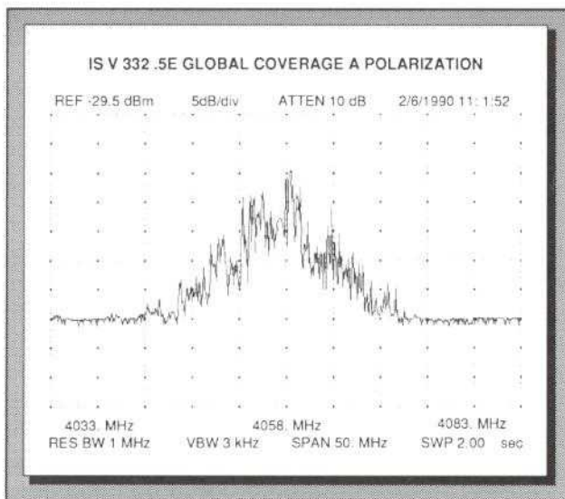
Figure 14. Typical AOR remote C-band monitor display at 30-MHz video carrier
