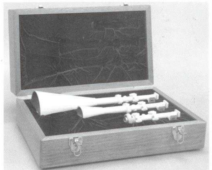
Figure 20. 20-GHz gain standard antennas for NIST
