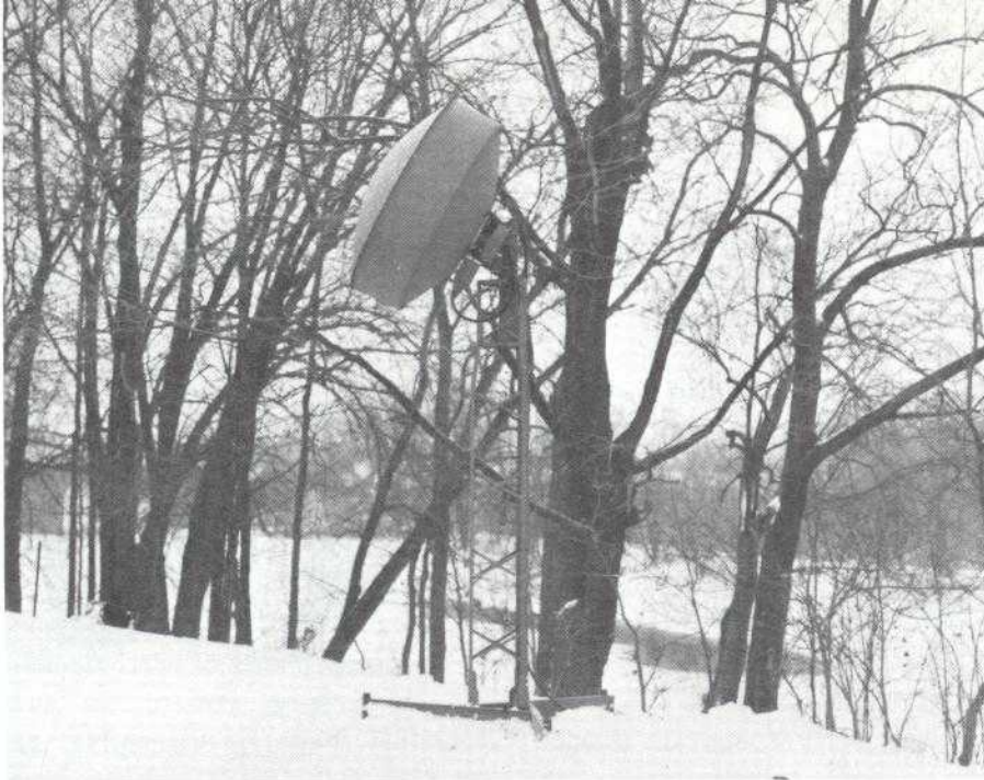
A small antenna transmits hydrological data by satellite to receive points in the United States and Canada.
